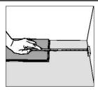
4 At the end of the first row, leave an expansion gap of %" to the wall and measure the length of the last plank to fit.
