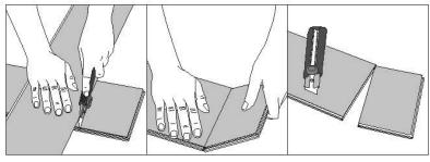
(§) To cut the plank, use a simple utility knife and ruler, and with he top side facing up, cut heavily and several times on the same axis. The knife will not go through the surface but make a deep cut. You can then lift one half of the plank using your other hand to hold down the second placing it very close to the cut. The plank will split naturally.
