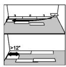
(§) Start the second row with the leftover cut part of the last plank of the previous row. This small plank should measure at least 12". Otherwise, use another plank that should be cut in two. The end joints of each adjoining row should not be closer than 10 the plant of the control of t
