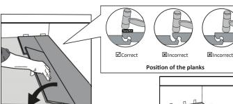
① Click the long side of the plank into the previous row and place it tight to the short end of the previous plank with an angle of 30 degrees. Lower the plank until it is resting in line with the adjacent plank. Firmly strike the surface of the locking mechanism with a Soft Faced Hammer and a tapping block until the planks are locked together at the same height. Make sure both planks are perfectly aligned.
