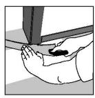
① Door molding and skirting: lay a board (with the decorative side down) next to the door molding and as shown in the figure. Then slide the floorboard under molding.
