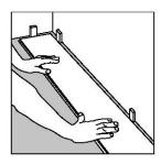
① After thoroughly cleaning the subfloor, you should begin laying in the left-hand corner. Place the floorboard %" from the left wall. Use spacers between the wall and the floorboard.
